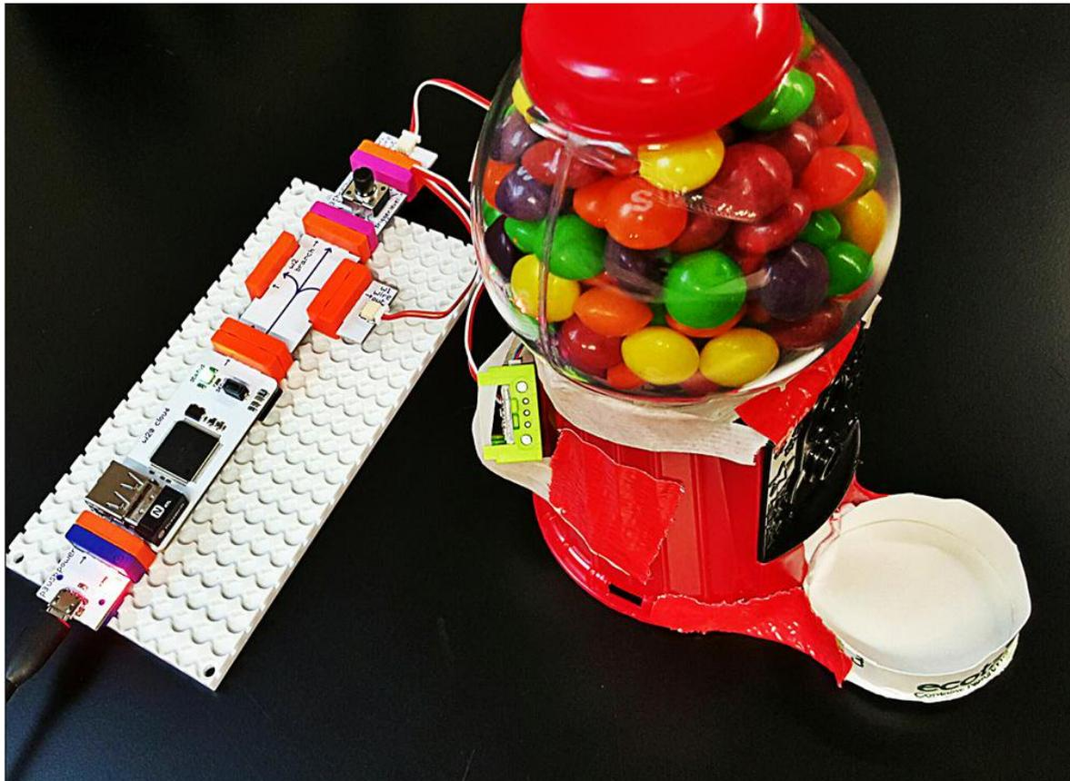
*Figure 4. Photograph of the Naughty or Nice sweet dispenser, an IoT object connected using littleBits and Slack.*
